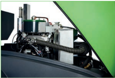
Heat exchanger for engine cooling with pre-heating from the water in the tank gives up to 15 % fuel saving
