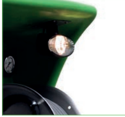
Light package:work light and beacon adjustable with joystick code: 1.229.240
